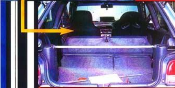
Fitting the rear bar required some modifications to the plastic trim
