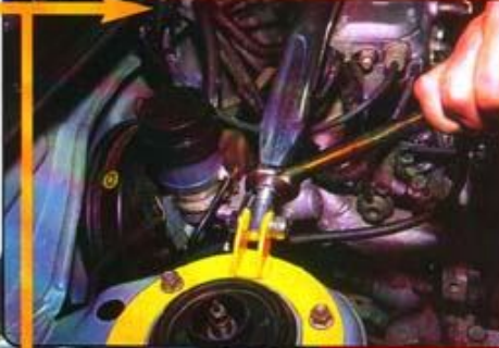
The final fitting. It is important not to pre-load the strut brace, or fit it while the car is jacked up. Doing this will dramatically reduce the effectiveness of the brace.
