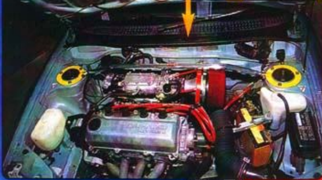
The final fitting. It is important not to pre-load the strut brace, or fit it while the car is jacked up. Doing this will dramatically reduce the effectiveness of the brace.
