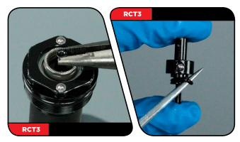
**RC Only:** Use needle-nose pliers to remove the bleed plug from the compression adjuster.
