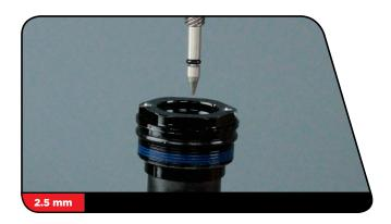
**19 RCT3 Only:** Insert the compression cam assembly into the bladder assembly and turn it clockwise to lock it into place.
