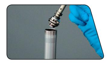
Spray isopropyl alcohol on the threads inside the coupler and clean the threads with a rag.
