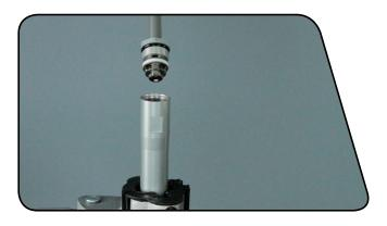
Place a torque wrench with a 21 mm crowfoot open end wrench on the wrench flats on the damper seal head. Place a 21 mm open wrench on the wrench flats of the cartridge tube.
