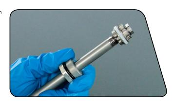
6 Lightly clamp the cartridge tube into a bicycle stand with the threads at the bottom and wrench flats at the top. Thread the rebound assembly into the cartridge tube by hand.
