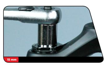
RC Only: Use a 15 mm socket wrench to turn the low speed compression adjuster clockwise until it stops.
