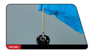
RCT3 Only: Use needle-nose pliers to grasp the wrench flats on the compression cam assembly. Pull the compression cam assembly out of the bladder assembly.
