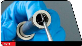
**RC Only:** Use needle-nose pliers to grasp the wrench flats on the compression adjuster. Pull the compression adjuster out of the bladder assembly.
