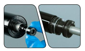
Spray isopropyl alcohol on the inside and outside of the upper tube and clean it with a rag.
