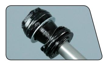
Firmly push the air shaft assembly into the bottom of the upper tube while gently rocking the air shaft side to side.
