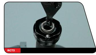
**RC Only:** Use small retaining ring pliers to remove the retaining ring from the bleed plug.
