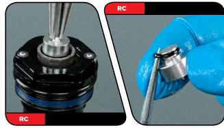
RCT3 Only: Use small retaining ring pliers to remove the retaining
