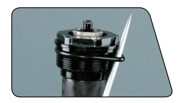
Clamp the cartridge tube into a bicycle stand with the rebound damper shaft oriented upward.
