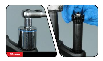
Use your fingers or a pick to remove the compression top cap o-ring.
