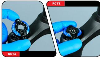
**RC Only:** Place the compression mode adjuster knob onto the compression top cap with the long tab near the **back** of the crown. Turn the compression mode adjuster **counter-clockwise** until it engages the first detent space.
