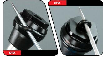
**Solo Air Only**: Use your fingers or a pick to remove the air piston quad ring.
