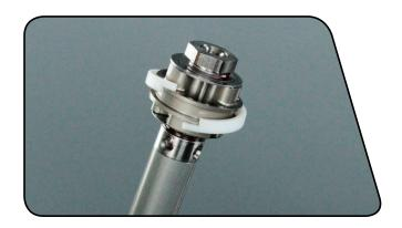
**9** Clamp the wrench flats of the coupler into a vice with the cartridge tube oriented upward.
