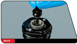
**RC Only:** Use needle-nose pliers to insert the bleed plug into the compression adjuster until it clicks into place.
