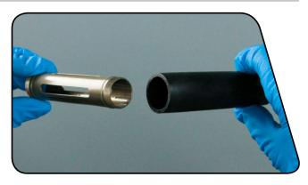
2 Apply a liberal amount of SRAM® Butter onto both ends of the bladder.
