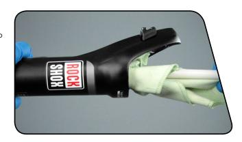
Reinstall new foam rings on the top bushings in the lower leg.
