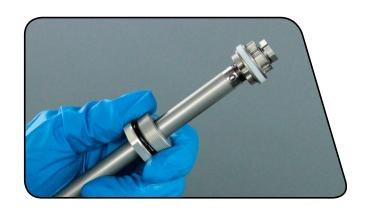
Use your fingers or a pick to remove the seal head o-ring. Use a pick to pierce and remove the scraper.
