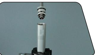
8 Remove the cartridge tube from the bicycle stand and pour the suspension fluid into an oil pan.
