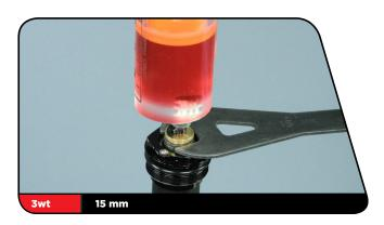
Create a vacuum in the damper assembly by pulling up on the syringe handle and simultaneously pushing up on the rebound damper shaft. This will force bubbles out of the damper assembly.
