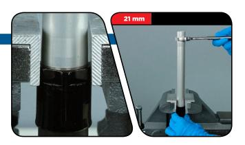
Remove the coupler, bladder, and compression top cap assembly from the vise.
