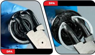
**Solo Air Only:** Use a flat blade screwdriver to push the SA seal head tab under the retaining ring.
