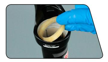
Remove the wire spring from the new dust wiper seal and set it aside.
