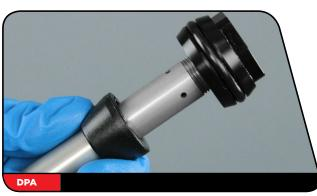
**Solo Air Only:** Install a new bumper cone with the broad base facing away from the SA piston.
