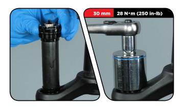
**RCT3 Only:** Use a 15 mm socket wrench to turn the compression cam assembly **counter-clockwise** until it stops.
