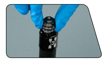
Use your fingers or a pick to remove the o-ring on the compression piston assembly.  $\,$
