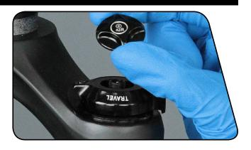
Use a small hex wrench to depress the Schrader valve and release all air pressure from the air chamber.
