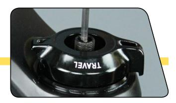
Use a 2.5 mm hex wrench to loosen the set screw and remove the rebound adjuster knob located at the bottom of the drive side fork leg.
