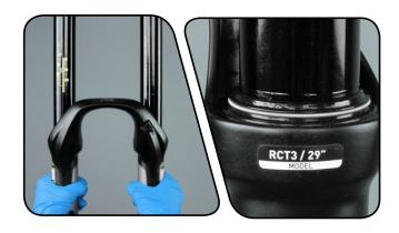
Position the fork at a slight angle with the bottom bolt holes oriented upward. Angle the syringe fitting in each lower leg bolt hole so as not to fill the shaft. Inject 5 mL of RockShox Ow-30 suspension fluid into the drive side leg, and 15 mL of RockShox Ow-30 suspension fluid into the non-drive side leg.
