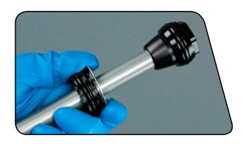
Use your fingers or a pick to remove the outer seal head o-ring. Use a pick to pierce and remove the inner o-ring and scraper.
