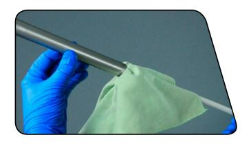
Install the seal head assembly onto the rebound damper shaft with the threads oriented toward the piston.
