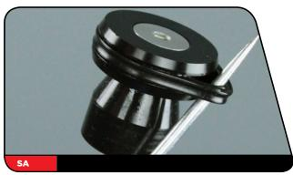
Use your fingers to remove the bumper cone from the air shaft.
