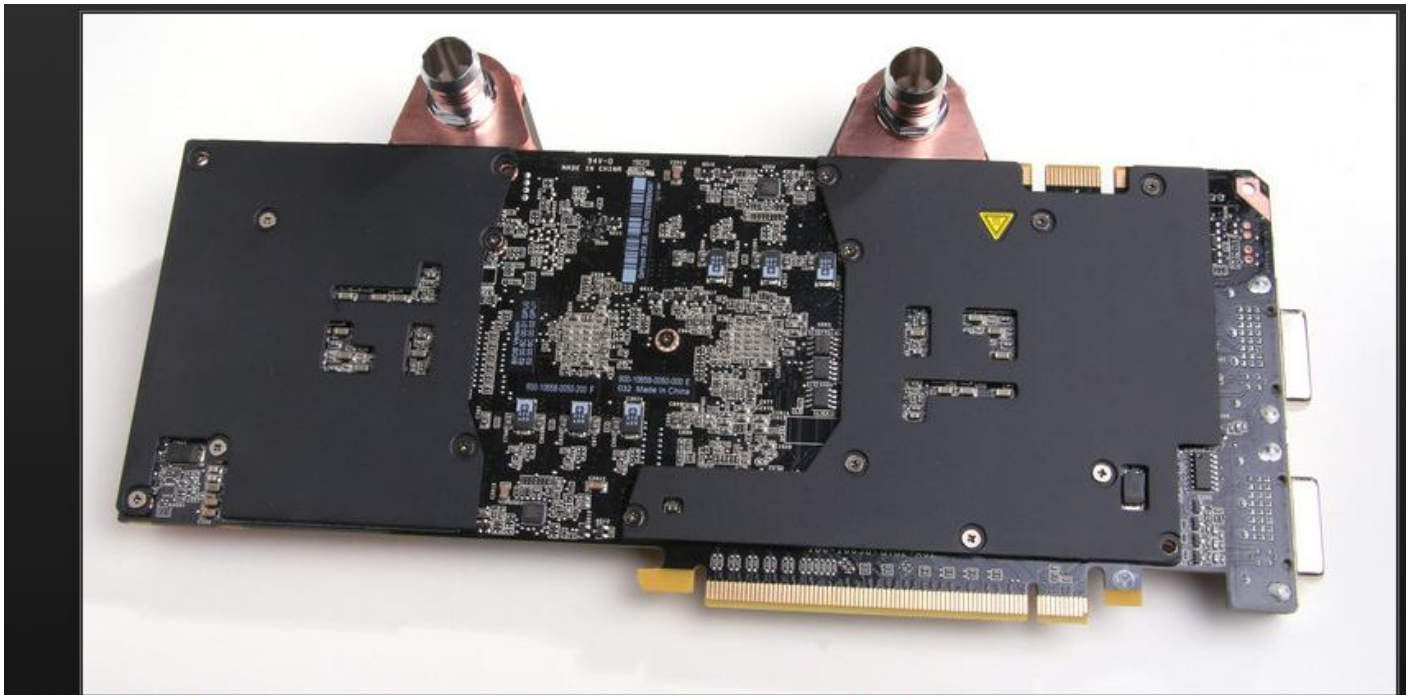
Slide the block under the card and place the backplates back on. Tighten the screws firmly.
