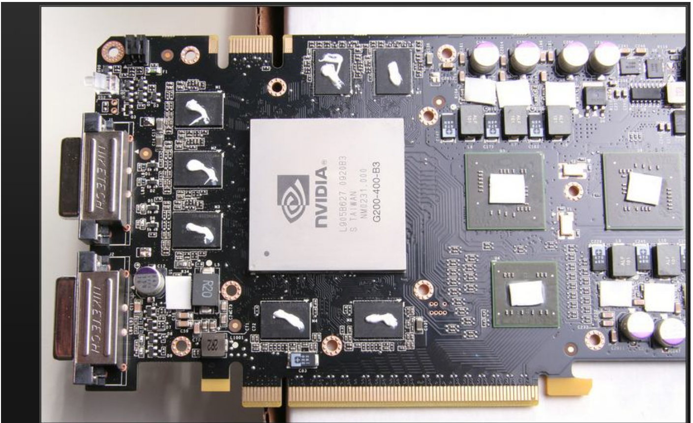
Locations for the thermal paste and thermal tape.
