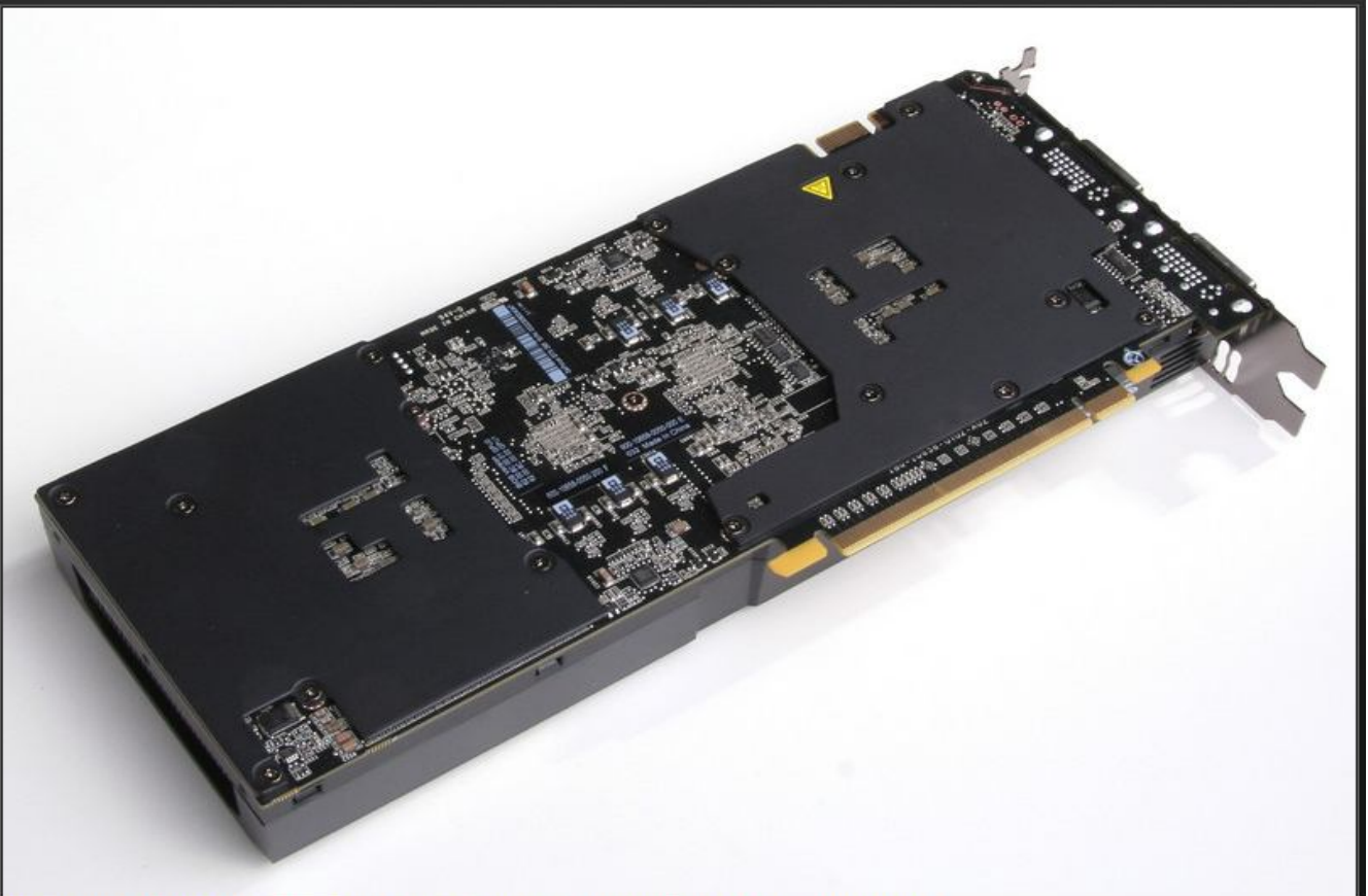
This backplate and all the screws get reused with the block installation. Be sure to save these!
