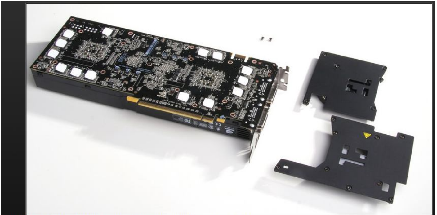
Now you can take the backplates off...remember to save them and the screws!
