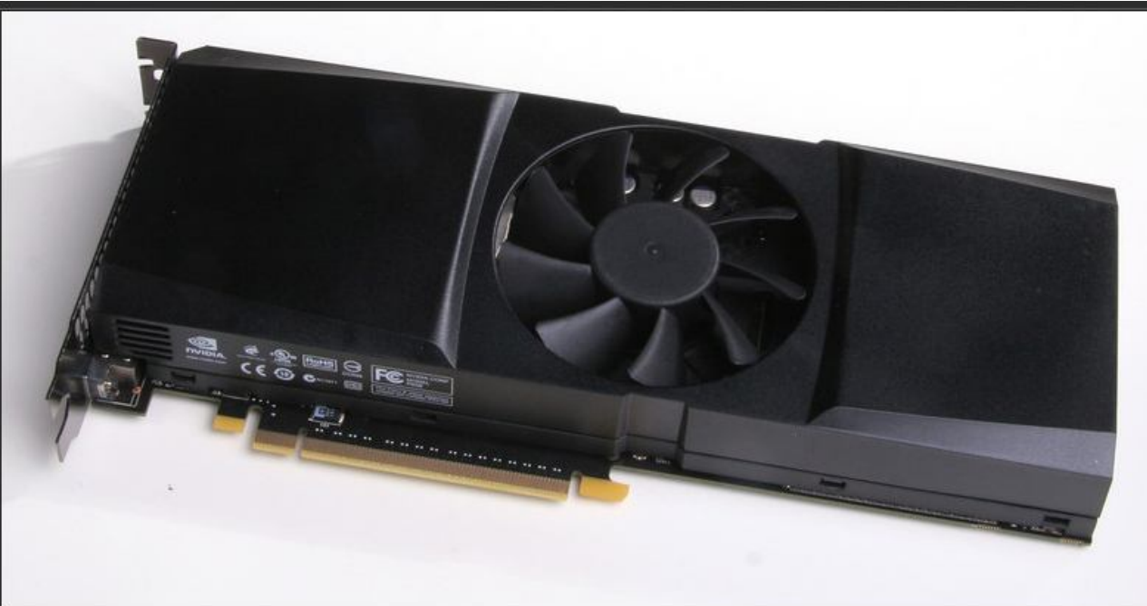
Nvidia OEM heatsink. To remove requires releasing the snaps on the sides and removing the screws.
