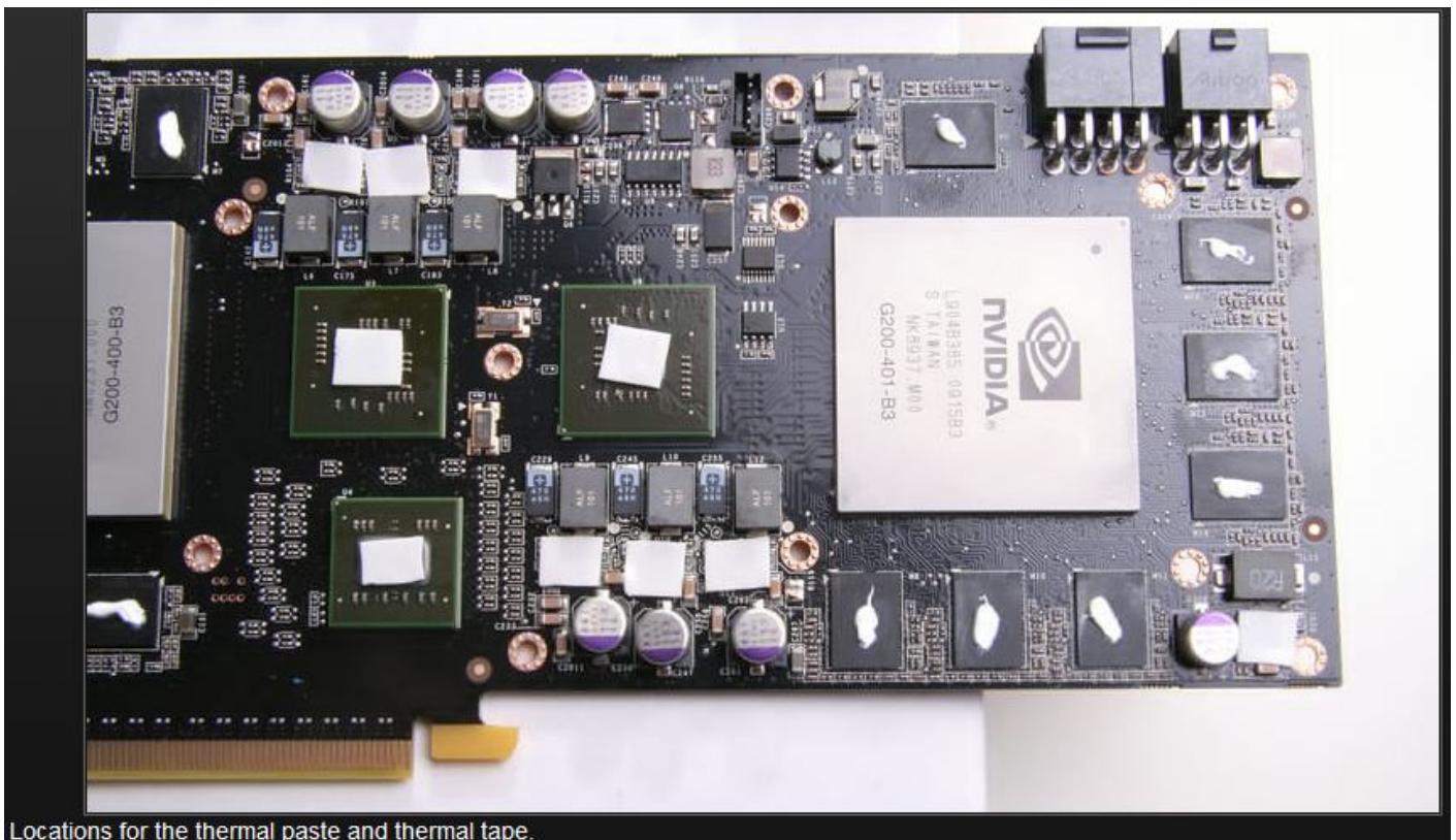
Locations for the thermal paste and thermal tape.
