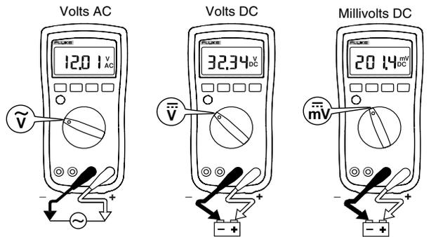
**Figure 1. Measuring AC and DC Voltage**
