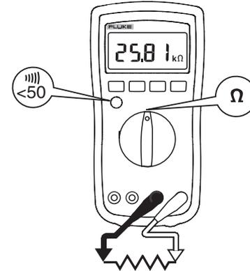
Figure 3. Measuring Resistance/Continuity
